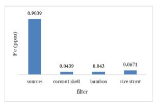
Figure 5. Fe filtration result using AAS.
