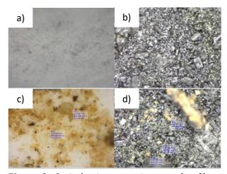
**Figure 3**. Optical microscope images of a filter paper (a), a filter paper with SMC material (b), the filter paper (c), and filter paper with SMC material (d) after being used for filtering the Mataram canal water samples.
