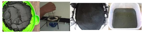
**Figure 2**. Treatments of the carbon materials. Heating the sediment obtained after ultrasonication (top left), the SMC material obtained after the heating process (top right), The SMC material dissolved in distilled water (bottom left), and the SMC as a filtration material on the filtration paper (bottom right).
